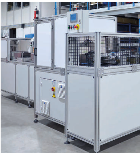
Protective device guard with interlocked swing doors for removal and inspection of the component
