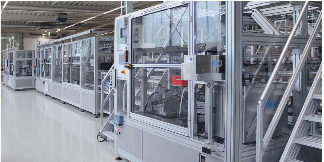
Protective housing for 45 metre long assembly system with passages and bridges for maintenance
