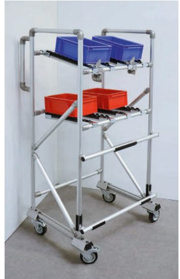
Kanban material provision station with rollers strips
