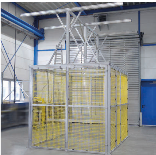
Guarding for transfer station with cantilevers for mounting an overhead conveyor
