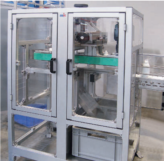
Guarding with swing doors made from cleanroom profiles
