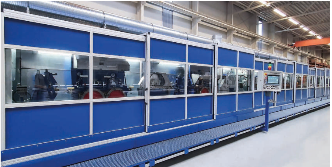
Mobile machine housing using Series 50 profiles for strip rolling line
