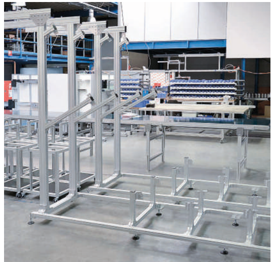
Frame for hopper conveyor made from Series 50 profiles
