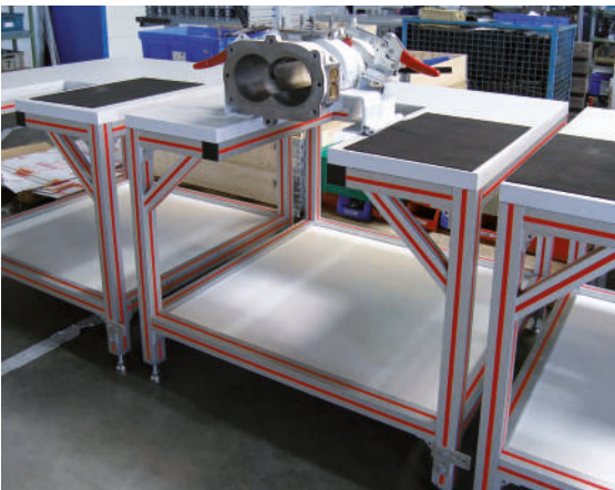
Assembly line for pumps built from Series 50 profiles with profile slots closed using red closure strips
