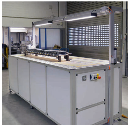
Assembly workstation with lowering mechanism based on electrically driven hydraulic cylinders
