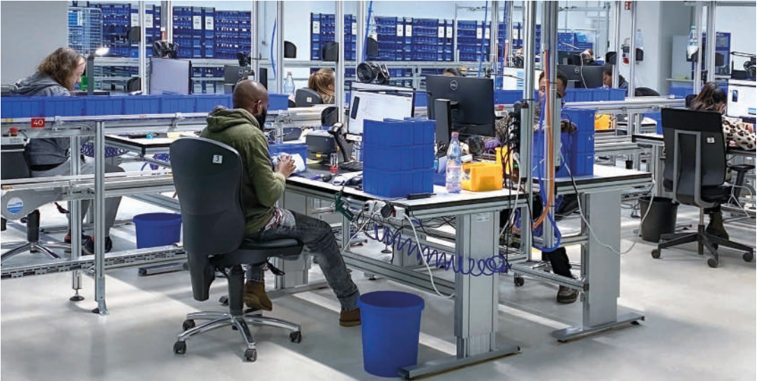
Workbench for manual inspection in the grading area for smartphones
