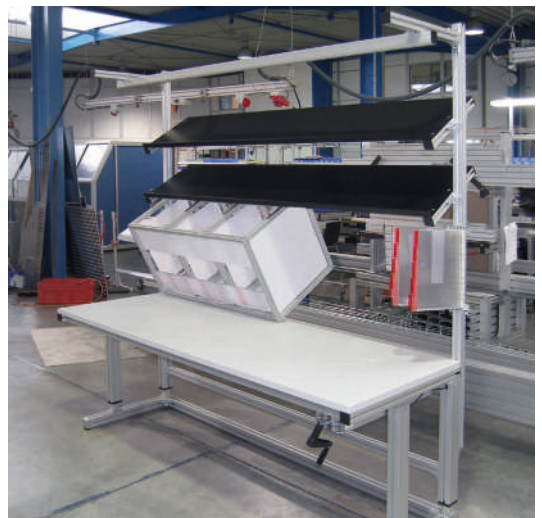
Workstation with hydraulic height adjustment and swivelling steel shelves with adjustable depth
