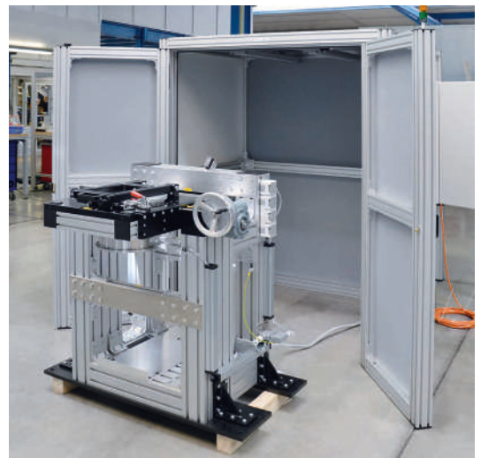
Protective housing for balancing stand, access via swing door with safety interlock and safety controller for the balancing stand
