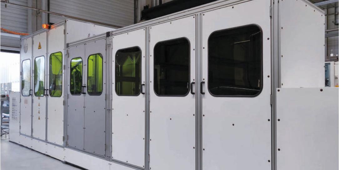
Protective laser enclosure with labyrinth seals for automation line
