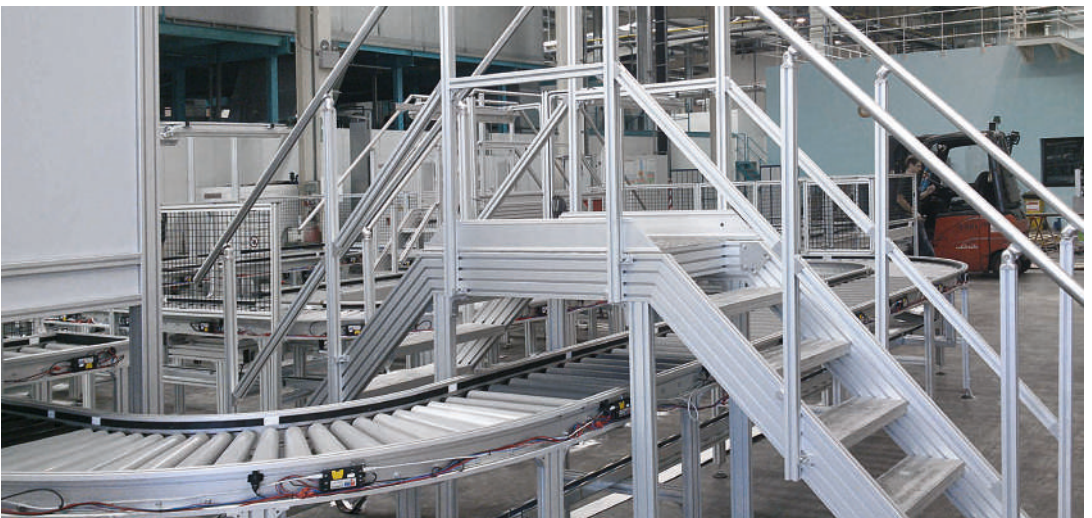
Free-standing bridge for bridging a conveying path in accordance with the regulations of the occupational health and safety directive (traffic routes)
