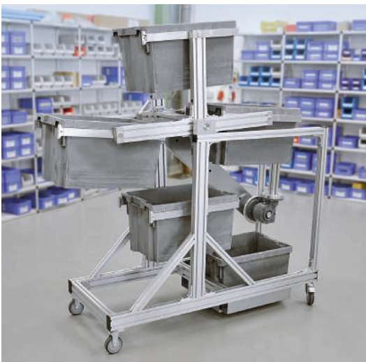
Material trolley for picking in narrow aisles with carousel concept
