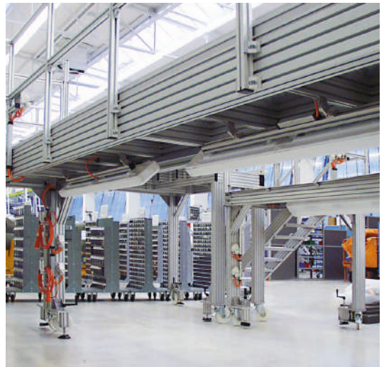
The T-slots are suitable for attaching components, such as the electrical supply
