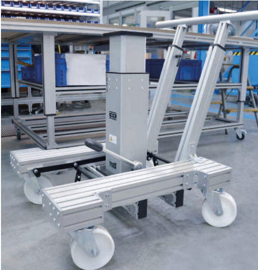
Assembly trolley with hydraulic cylinder and central locking device
