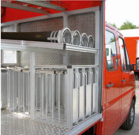
Fire engine interior built from Series 25 profiles
