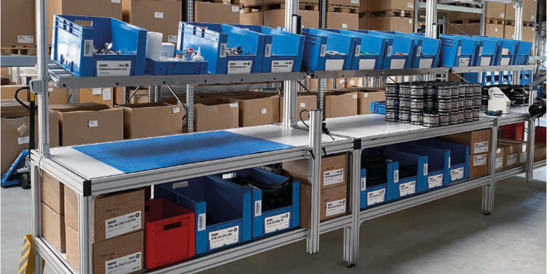
Stable assembly workstations with profile racks and shelves
