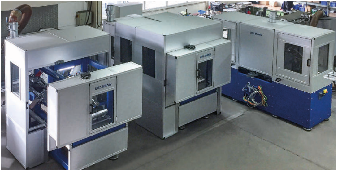
Extendible guarding elements; sections mounted on rollers can be moved manually over the first section
